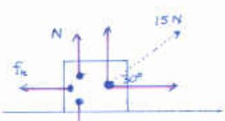
$$\text{Solve for } \mu_k: -\mu_k(21.9 \text{ N}) = 7.8 \text{ N} - (15 \text{ N})\cos 30^\circ = -5.19 \text{ N} \rightarrow \mu_k = 0.237$$
