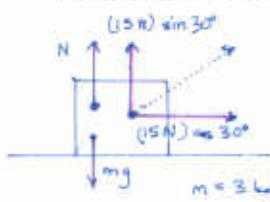
Forces on the block are as shown here with the 15 N force resolved into components. There is no net vertical force only a net horizontal force which is
