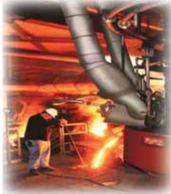
High efficiency Cupola capable of 60 tons per hour
